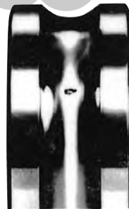
Fig. 5.1 Example of Flaking
